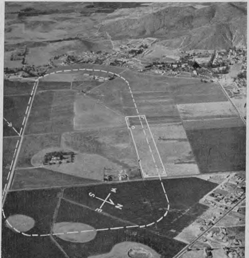
LA SIERRA AIRSTRIP AND TRAFFIC PATTERN — Solid line outlines flight strip, 300x1800 feet. Dashed line indicates traffic pattern, which is always to south of strip at 600 feet. West pattern is left hand, east pattern right hand. With no wind, pattern is always flown to the West. CAUTION — 35 ft. hi-voltage line across east end of strip. If interested in regulations governing strip write Physics Department, LSC.
