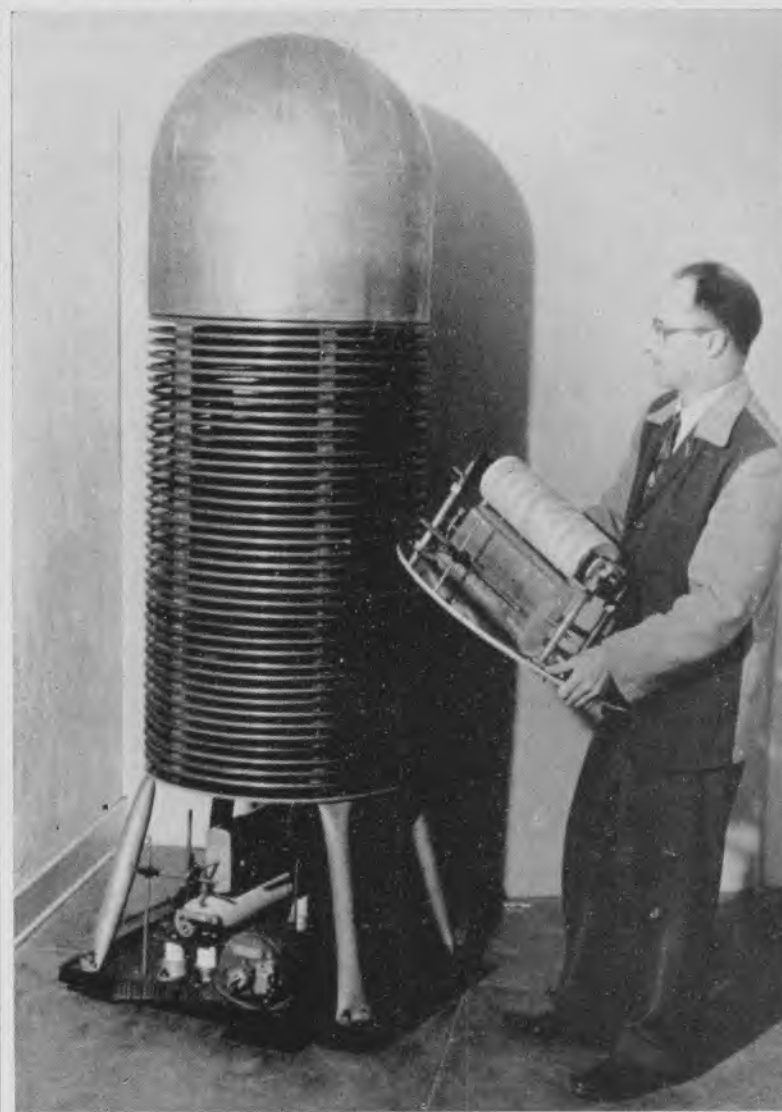
James Riggs, instructor in physics, holds the idler pulley which fits under the dome of the Van de Graff electrostatic generator which he has constructed for demonstration in the LSC physics department.
