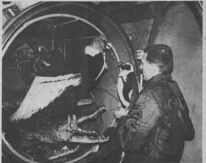
Elmer Hankins places several animals into the freeze-dry unit so they will be preserved.
